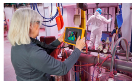
Portable acoustic imager detects leaks
