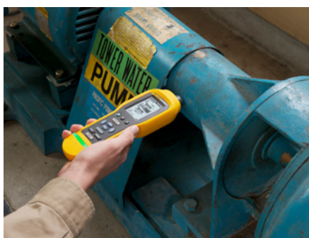
Overall vibration levels for screening and trending using the Fluke-805
