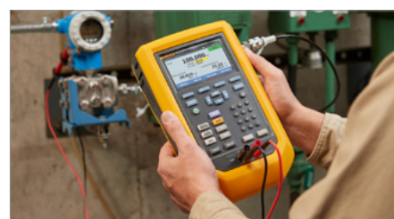
Portable automatic pressure calibration
